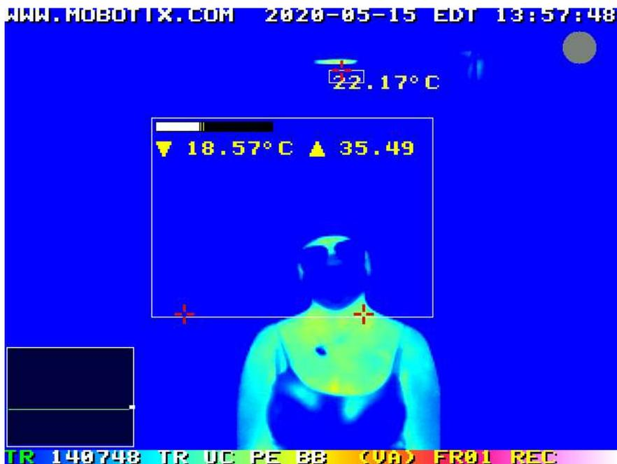
Note: The MOBOTIX Thermographic cameras TR will measure the hottest pixel in the area of measurement. The carotid artery temperature is reflected in the measurement on the neck area.
